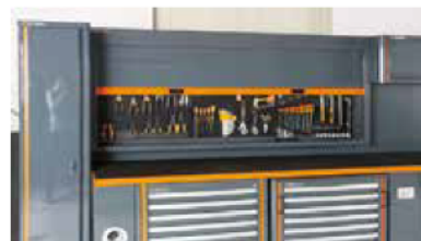
Aluminium shutter with lock for protecting tools
