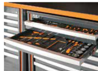
Drawers can accommodate thermoformed tool trays
